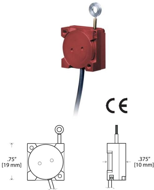
Introducing the world's smallest stringpot. The M150 is smaller than a thumbprint and occupies a tiny space of only .74 x .74 x .38 inches. With a full stroke measurement range of 1.5 inches, the M150 has been designed for many aerospace and automotive space-critical test applications such as throttle position and crash-test instrumentation.
