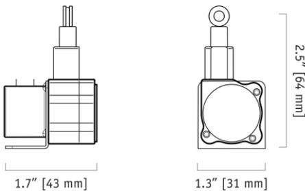
With its ultra-compact design the SM1 is the perfect solution when tight space is an issue. At just a little over an inch across, this miniature stringpot offers full stroke measurement ranges from 2½ to 25 inches. A precision plastic hybrid 10K-ohm potentiometer delivers a precise voltage divider output signal that is linearly proportional to the travel of the spring-loaded measuring cable.
